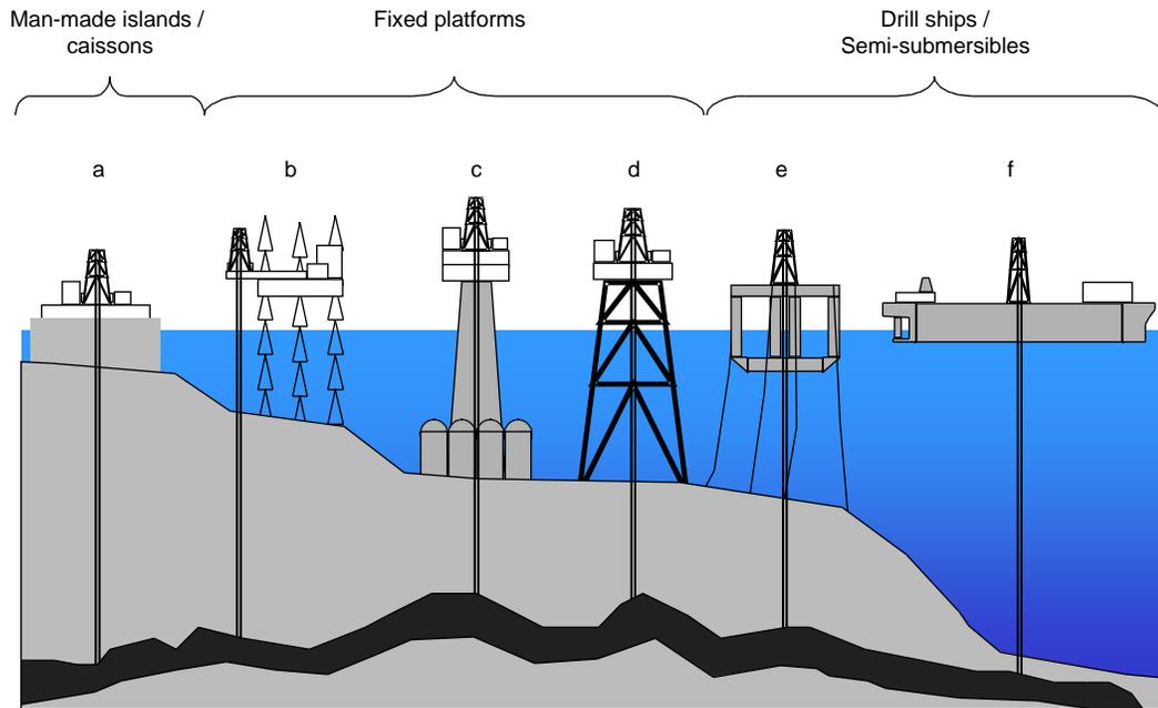
Figure 3.2. Common oil and gas rig and platform types, (a) Man-made island, (b) Jack-up rig, (c) gravity based structure, (d) metal jacket, (e) semi-submersible rig, (f) drill ship.
